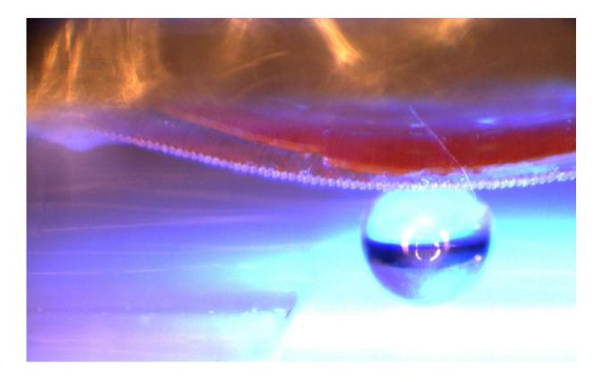
When illuminated with UV light, the intelligent material with the adhesive surface bends. This way it can lift, transport and put down flat and threedimensional objects (here, a 1 millimetre diameter glass sphere). Credit: Emre Kizilkan
