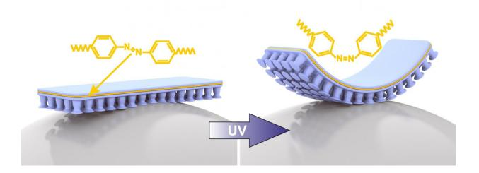
The azobenzene molecular structure re-configures when exposed to UV light, bending the sticky structure until attached items fall off. Credit: Emre Kizilkan and Jan Strueben
