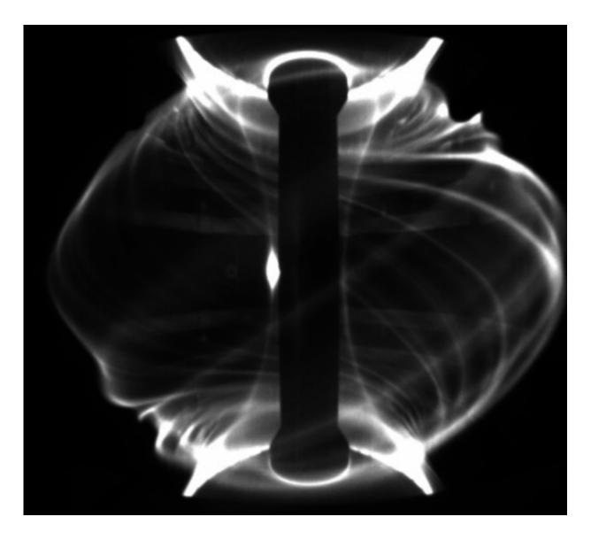
Here you can see the twist in the plasma within a tokamak. Credit: CCFE
