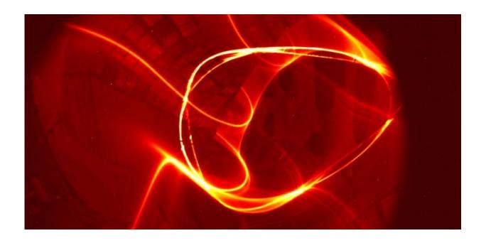
The superheated plasma inside the fusion reactor is twisted by magnetic fields. Credit: IPP, Matthias Otte
