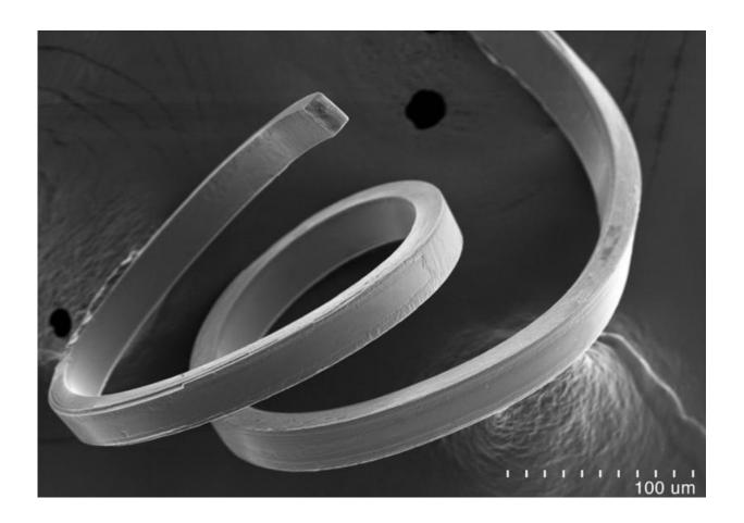
A scanning electron microscopy image of flexible haloimidazole crystals, which were found to show both ferroelectric and piezoelectric properties. Credit: Seungbum Hong/Argonne National Laboratory
