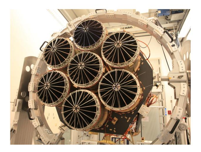
After about ten years of development and integration the eROSITA X-ray telescope is complete: with 7 mirror modules and 54 mirror shells each combined with 7 specially built X-ray cameras. You see the telescope here after final integration at MPE, shortly before transport to further testing. Credit: MPE
