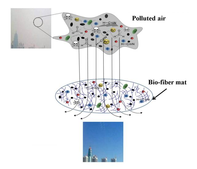
WSU's new soy-based filter is able to capture challenging pollutants from the atmosphere. Credit: WSU
