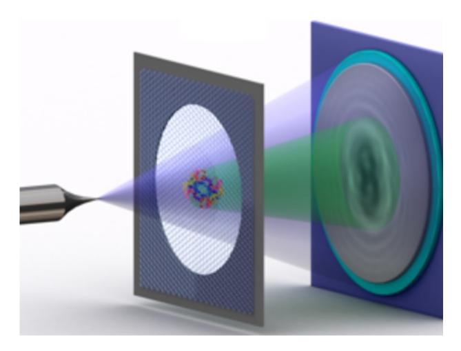
Diagram showing the electron holography of single proteins: A metal tip whose end tapers to just a few atoms emits a beam of relatively slow, i.e., low-energy electrons. Part of the beam is scattered by the protein on a graphene carrier. The scattered part of the beam then generates an interference pattern with the nonscattered part – the hologram – which is recorded. Credit: Tatiana Latychevskaia /University of Zurich
