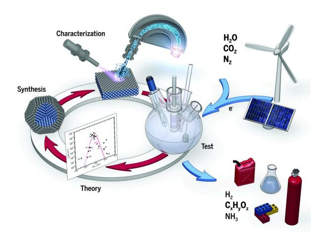
Schematic showing electrochemical conversion of water, carbon dioxide, and nitrogen into value-added products (e.g., hydrogen, hydrocarbons, oxygenates, and ammonia), using energy from renewable sources. The combination of theoretical and experimental studies working in concert provides us with insight into these electrochemical transformations and guides the development of the high-performance electrocatalysts needed to enable these technologies. Credit: Jakob Kibsgaard, DTU Physics
