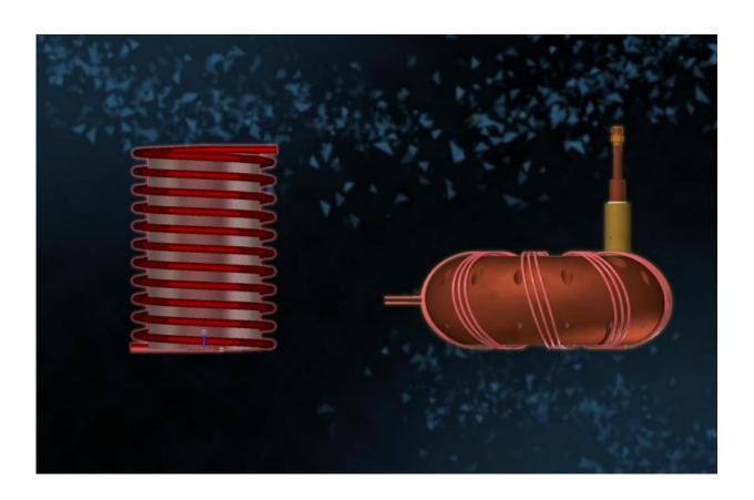
Scientists at IBS CAPP are prototyping haloscopes - machines that hunt for dark matter. Haloscope have very strong magnets. Helix-shaped magnets (solenoid magnets, on the left) are commonly used in dark matter experiments. CAPP scientists are also investigating the possibility of using donut-shaped magnets, technically known as toroidal magnets, and nicknamed this device the CAPPuccino submarine. Credit: Institute for Basic Science
