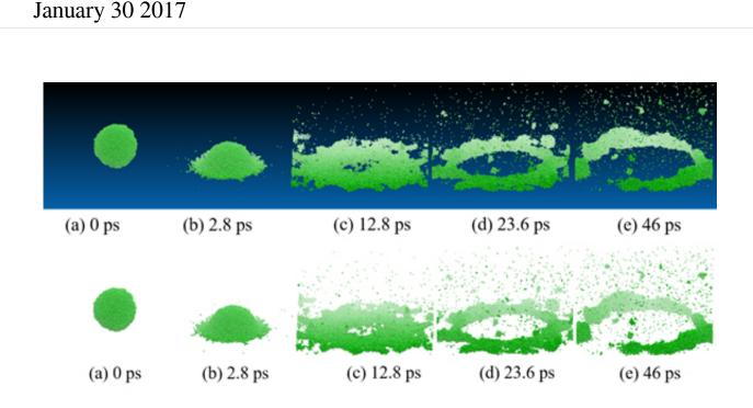
These figures show how a nanodroplet breaks up when it impinges on the solid wall through molecular dynamic simulation in computer. There are 12,195 water molecules represented by the green particles in this figure (the droplet originally has a diameter of 8.6 nm). Credit: Li, Li and Chen
