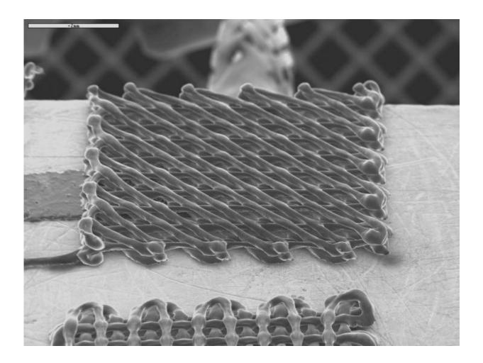
As soon as it comes out of the printing nozzle, the solvent evaporates and the ink solidifies. It takes the form of filaments slightly bigger than a hair. The manufacturing work can then begin. Credit: Polytechnique Montréal
