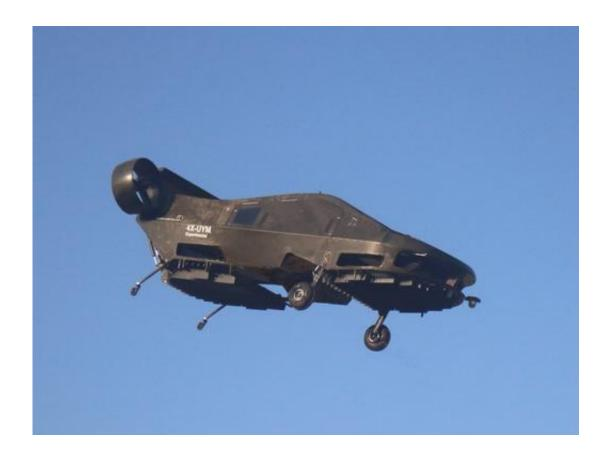
This image provided by Urban Aeronautics/Tactical Robotics shows an Israelimade flying car. Urban Aeronautics conducted flight tests of its passenger-carrying drone call the Cormorant in Megiddo, Israel, late in 2016. The company says the aircraft can fly between buildings and below power lines, attain speeds up to 115 mph, stay aloft for an hour and carry up to 1,100 pounds. (Urban Aeronautics/Tactical Robotics via AP)
