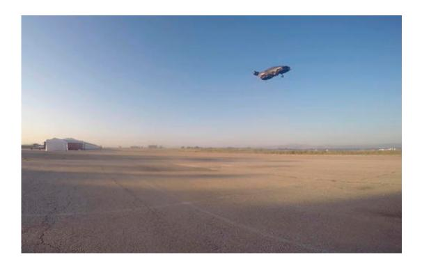
This image provided by Urban Aeronautics/Tactical Robotics shows an Israelimade flying car. Urban Aeronautics conducted flight tests of its passenger-carrying drone call the Cormorant in Megiddo, Israel, late in 2016. The company says the aircraft can fly between buildings and below power lines, attain speeds up to 115 mph, stay aloft for an hour and carry up to 1,100 pounds. (Urban Aeronautics/Tactical Robotics via AP)
