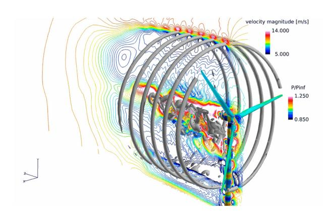
From a simulation run on the Yellowstone supercomputer, these contour lines and isosurfaces provide valuable information about turbulence and aerodynamic drag in this visualization of air flow through the blades of a wind turbine. Credit: Dimitri Mavriplis, University of Wyoming
