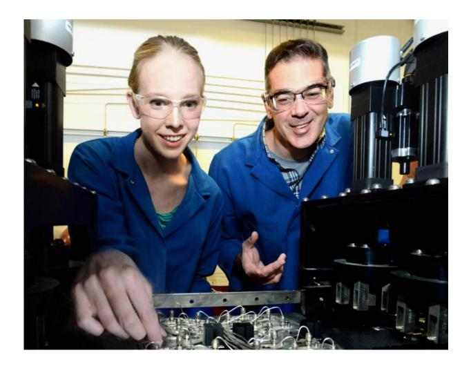
Jeffrey Long and graduate student Kristen Colwell will use a custom-built device to analyze CO2 uptake from a simulated flue gas. More than two dozen samples can be analyzed at a time. Credit: Peg Skorpinski.
