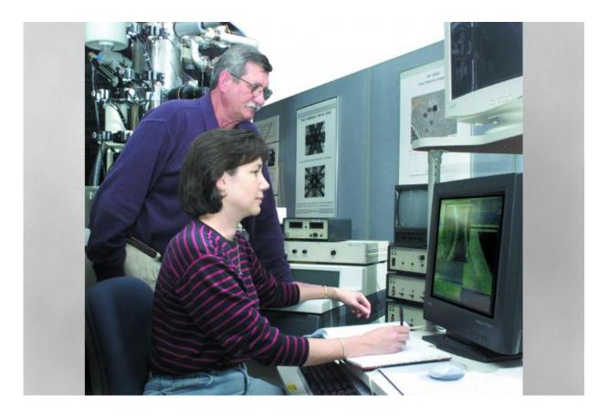
During DOE programs to advance industrial ceramic matrix composites, ORNL's Karren More (foreground, with Larry Walker) used transmission electron microscopy and other techniques to pinpoint causes of failure in stresstested or field-tested materials made by companies. Without the expertise and facilities of national labs—available nowhere else—industry would have been flying blind. Credit: Oak Ridge National Laboratory, U.S. Dept. of Energy
