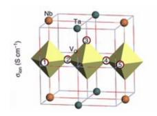
A schematic of the minimum energy migration pathway for an oxygen vacancy (VO) in SrCo0.75Nb0.125Ta0.125O3-δ, where dopants shown by coloured balls and Co along the pathway are within the octohedra. Other Co and Sr ions are omitted for clarity. The numbers 1–5 indicate the sequential positions of an oxygen vacancy along the diffusion pathway. Credit: Australian Nuclear Science and Technology Organisation (ANSTO)
