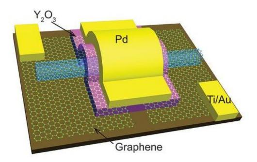
Schematic diagram showing the structure of a GC CNT FET. Credit: (c) *Science* (2017). DOI: 10.1126/science.aaj1628
