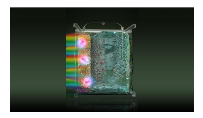
This is a schematic illustration of a photoelectrochemical cell for water splitting. The absorption of photons on the photoanode (left) generates electron and hole carriers. The electrons will flow through the circuit to the photocathode and evolve hydrogen (right), while the holes will evolve oxygen (left). Credit: Peter Allen/The Institute for Molecular Engineering, University of Chicago
