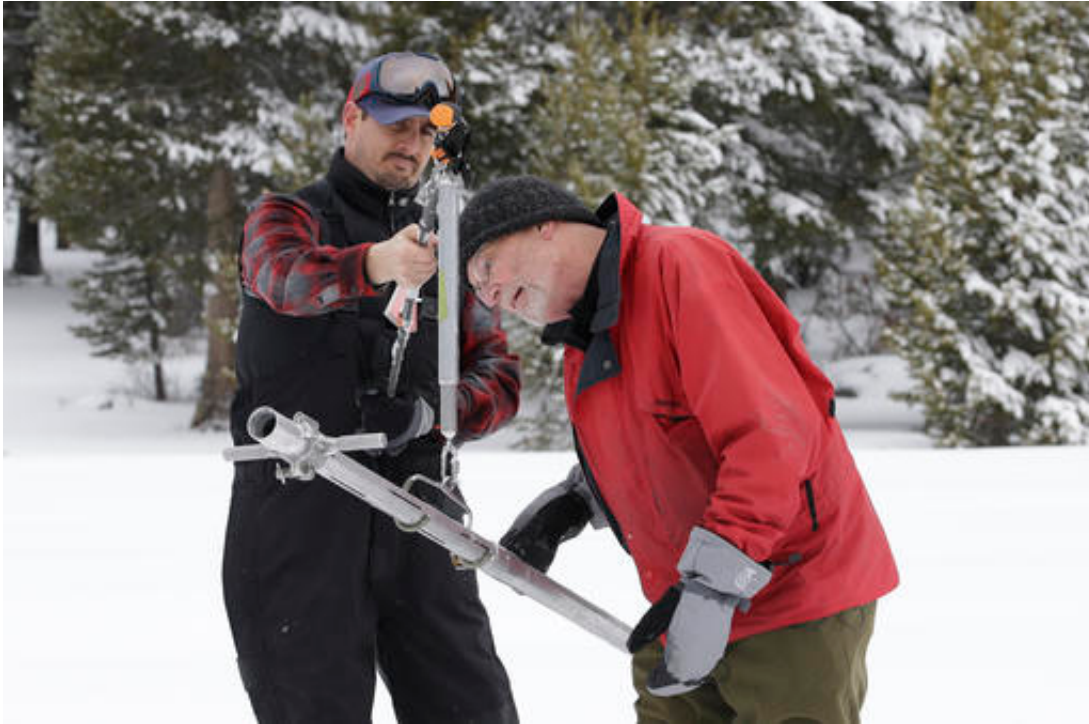
Frank Gehrke, right, chief of the California Cooperative Snow Surveys Program for the Department of Water Resources, checks the snowpack weight on a scale held by John Paasche, of DWR, during the first snow survey of the season at Phillips Station Tuesday, Jan. 3, 2017, in Echo Summit, Calif. The survey showed the snowpack at 53 percent of normal for this site at this time of year. (AP Photo/Rich Pedroncelli)
