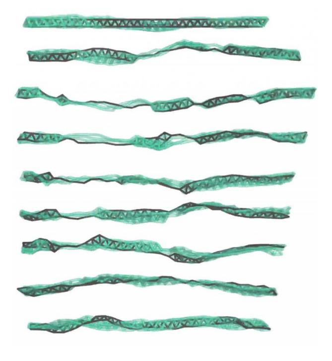
A simulation of one-dimensional boron under stress shows the theoretical material changing phase from a ribbon to a chain of atoms when pulled. The chain returns to ribbon form when the stress is relieved. Credit: Yakobson Group/Rice University
