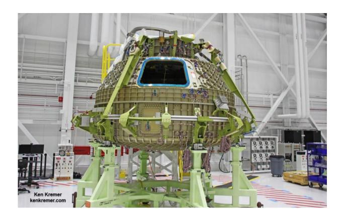
Hull of the Boeing CST-100 Starliner Structural Test Article (STA)- the first Starliner to be built in the company's modernized Commercial Crew and Cargo Processing Facility high bay at NASA's Kennedy Space Center in Florida. Credit: Ken Kremer/kenkremer.com
