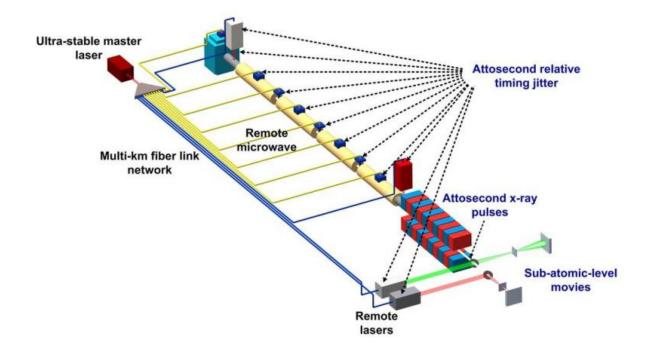
Schematic of the facility-wide synchronisation. Credit: DESY/Ming Xin
