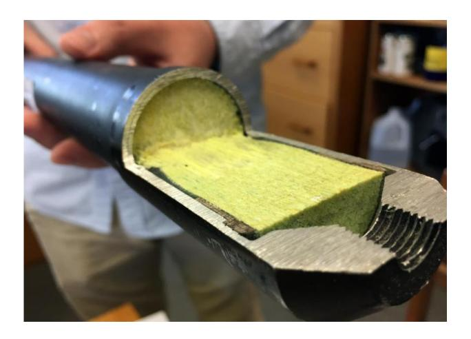
This hollow fiber module allows compression of a large surface volume, facilitating scalability. Credit: John Toon, Georgia Tech
