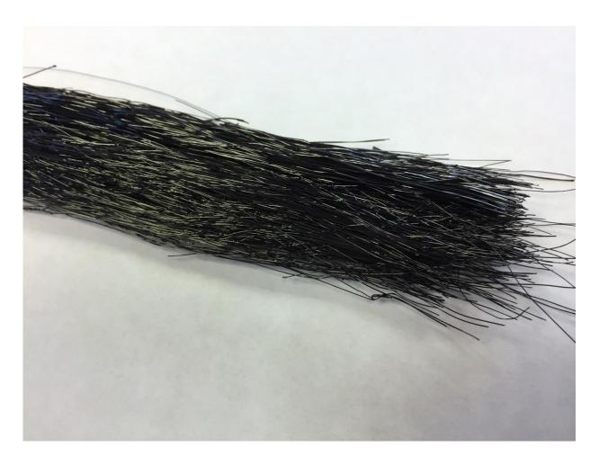
Carbon molecular sieve hollow fiber membranes are among the options for advanced separation technologies. Credit: John Toon, Georgia Tech
