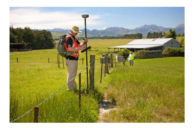
University of Michigan postdoctoral researcher Timothy Stahl uses GPS technology to measure displacement of a fence in New Zealand following November's magnitude-7.8 earthquake. Fence posts in the mid-ground were moved to the right by motion of the fault during the earthquake. Credit: Kate Pedley
