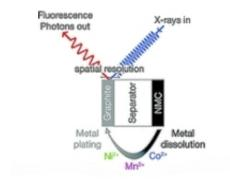
Operando X-ray spectroscopy set-up. Credit: HIMS
