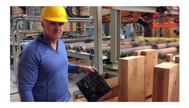
In this Nov. 11, 2016 photo, John Redfield, chief operating officer of D.R. Johnson Lumber Co. in Riddle, Ore., poses for a photo as he shows an example of a cross-laminated timber, or CLT, panel that underwent a flammability test. D.R. Johnson is one of just two companies in the United States currently able to produce CLT panels. (AP Photo/Gillian Flaccus)
