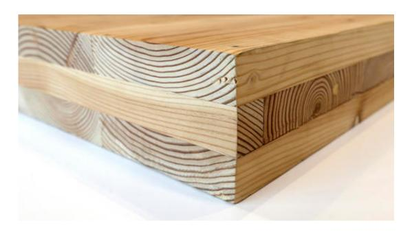
This Nov. 15, 2016, photo shows a piece of cross-laminated timber, or CLT, in Portland, Ore. CLT is made up of 2-by-4 beams laid out in perpendicular layers that are then glued together to make giant panels. (AP Photo/Don Ryan)
