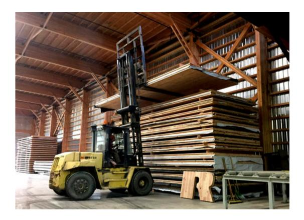
In this Nov. 11, 2016 photo, a forklift driver moves a newly assembled panel of cross-laminated timber, or CLT, to a stack in the production facility of D.R. Johnson Lumber Co., in Riddle, Ore. D.R. Johnson is one of just two companies in the United States currently able to produce CLT panels. (AP Photo/Gillian Flaccus)
