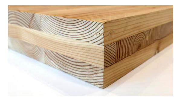
This Nov. 15, 2016, photo shows a piece of cross-laminated timber, or CLT, in Portland, Ore. CLT is made up of 2-by-4 beams laid out in perpendicular layers that are then glued together to make giant panels. (AP Photo/Don Ryan)
