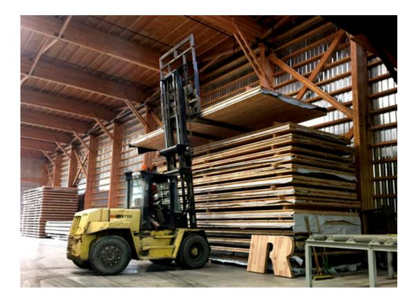
In this Nov. 11, 2016 photo, a forklift driver moves a newly assembled panel of cross-laminated timber, or CLT, to a stack in the production facility of D.R. Johnson Lumber Co., in Riddle, Ore. D.R. Johnson is one of just two companies in the United States currently able to produce CLT panels. (AP Photo/Gillian Flaccus)
