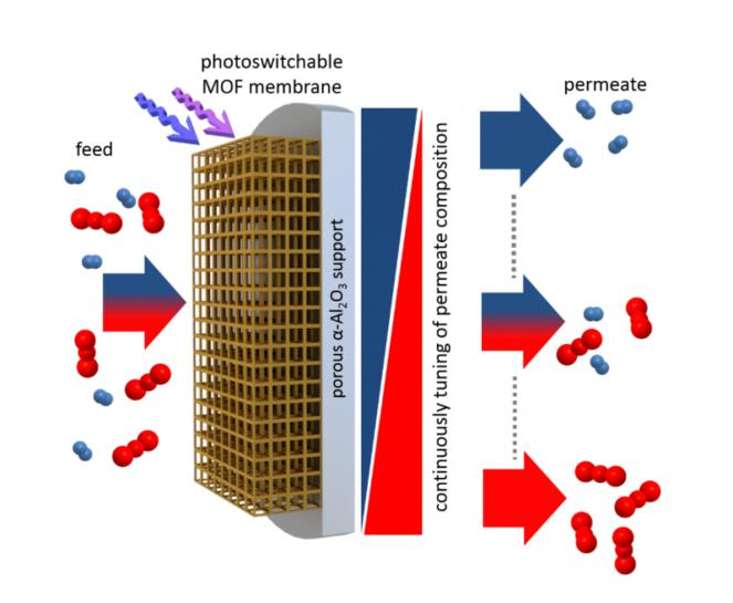
A MOF membrane with integrated photoswitches separates molecules. The separation factor can be tuned dynamically by light irradiation. Credit: Alexander Knebel/Universität Hannover and Lars Heinke/KIT
