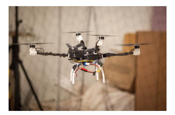
A four-rotor "bunnycopter" developed at MIT's Computer Science and Artificial Intelligence Laboratory features propellers at different heights. Credit: Jason Dorfman/MIT CSAIL
