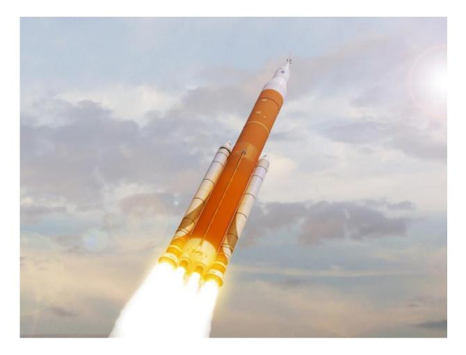
The next generation of NASA's Space Launch System will be 364 feet tall in the crew configuration, will deliver a 105-metric-ton (115-ton) lift capacity and feature a powerful exploration upper stage. On SLS's second flight with Orion, the newer rocket will carry up to four astronauts on a mission around the moon, in the deep-space proving ground for the technologies and capabilities needed on NASA's Journey to Mars. Credit: NASA
