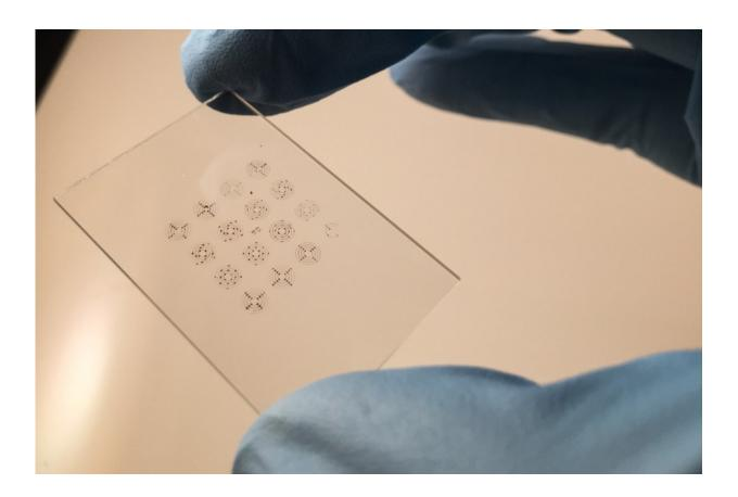
MIT researchers have fabricated a stamp made from forests of carbon nanotubes that is able to print electronic inks onto rigid and flexible surfaces. Credit: Sanha Kim and Dhanushkodi Mariappan
