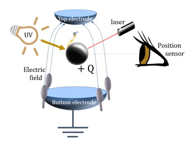
Electrostatic levitation. The UV source causes the metal to be ionized, giving it an electric charge and causing levitation in between the electrodes. The laser melts the metal. The new project involves electromagnetic in stead of electrostatic levitation. Credit: University of Twente
