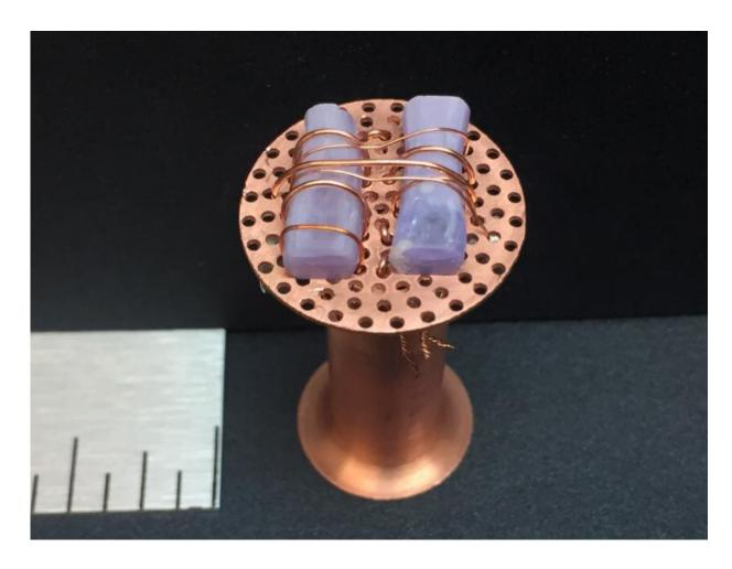
The tiny YbMgGaO4 crystal was reproduced by physicists at the University of Tennessee. The crystal, here perched on a stand for testing, appears to be the next extremely rare material to house an equally as rare observable quantum spin liquid. Credit: Georgia Tech / Martin Mourigal
