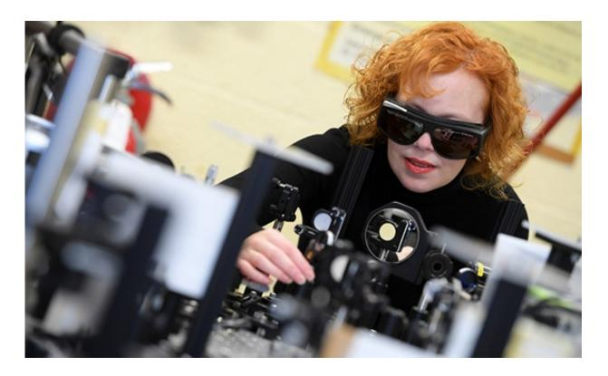
Dr. Kimberley Hall used ultrafast lasers in her lab to examine the exciton particles of perovskite, an emerging solar cell material. Credit: Danny Abriel
