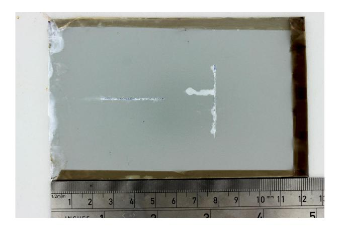
A steel panel with the new anti-corrosion treatment, after being exposed to hundreds of hours of salt spray, and showing virtually no signs of corrosion. Credit: Swansea University
