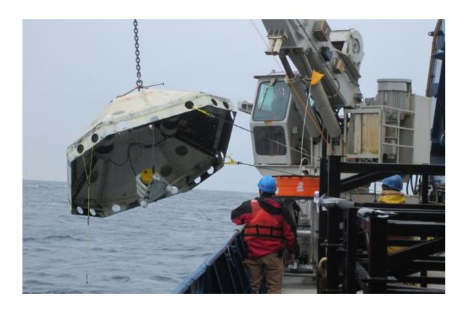
A ship-board crane lifts a Lamont-built ocean bottom seismometer attached to a protective trawler shield. Credit: Lamont-Doherty Earth Observatory
