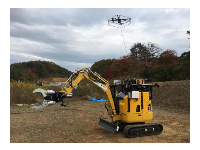
Rescue robot with a drone. Credit: Osaka University
