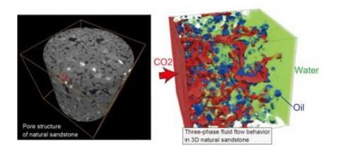
The pore geometry of natural sandstone (digital rock)was obtained using highresolution CT device (left), and CO2-water-oilbehavior within the heterogeneous pores were calculated usingthree-phase lattice-Boltzmann model (right). The greater detailprovided by the digital rock model simulation can help to identify therelevant processes of CO2 movement in oil reservoir and the rock'spotential for CO2 storage in natural rock. Credit: *Water Resources Research*
