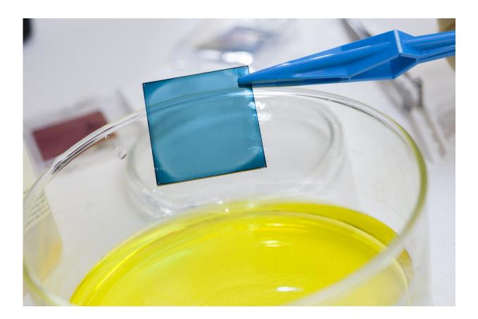
Close-up of a polymer film on a glass substrate before immersion in a polyoxometalte solution to electrically dope the film over a limited depth. Credit: Christopher Moore, Georgia Tech
