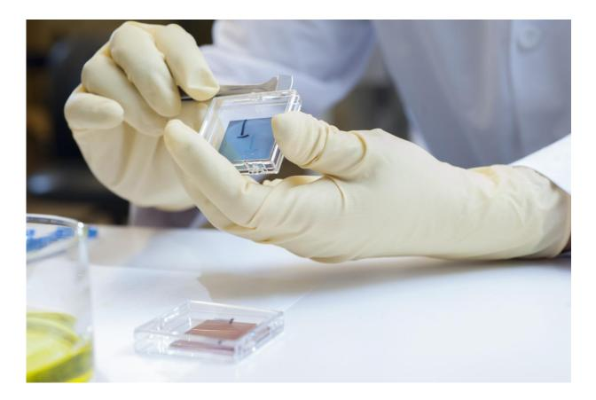
Close-up of polymer films used in polymeric solar cells doped by the new solution-based electrical doping technique. Credit: Christopher Moore, Georgia Tech
