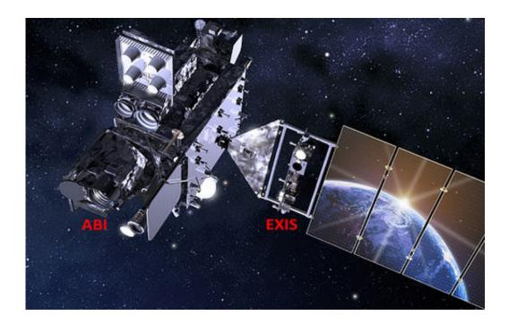
Artist's conception of the GOES-R satellite, showing the location of the two instruments tested and calibrated by NIST – the Advanced Baseline Imager (ABI) and the Extreme Ultraviolet and X-Ray Irradiance Sensor (EXIS). Credit: NASA
