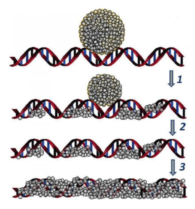
(1) A silver nanoparticle interacts with a DNA molecule. (2) The metal particle breaks up into smaller structures called nanoclusters. (3) Silver nanoclusters are distributed evenly along the double helix due to diffusion. Credit: Moscow Institute of Physics and Technology
