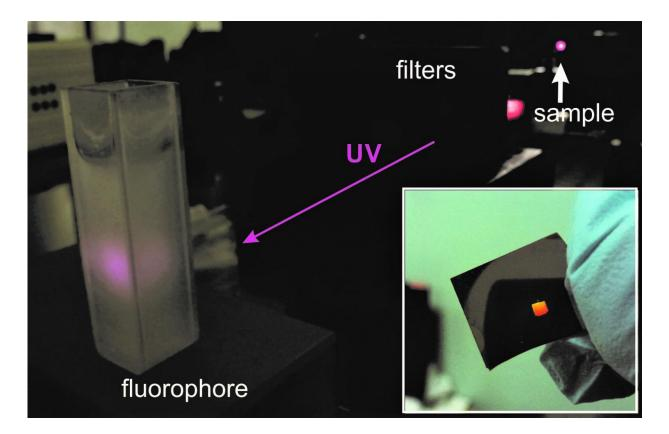
Photography of fluorescence induced by generated UV light in fluorophore. Inset - view of the sample with a self-organized metasurface (orange area). Credit: ITMO University
