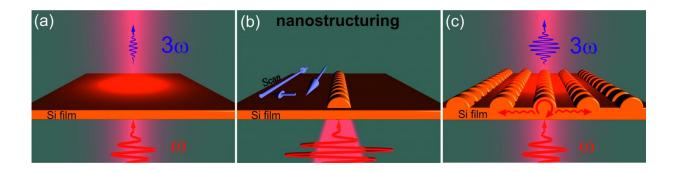
Schematic sketches of UV generation from (a) smooth and (c) nanostructured Si film. (b) Principle of Si film laser-induced nanostructuring. Credit: ITMO University
