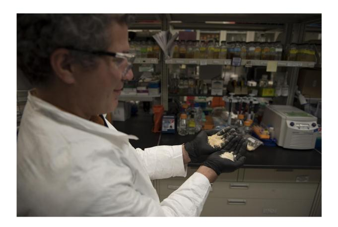
PNNL microbiologist George Bonheyo displays the original sawdust material (left) and how it appears after being chemically modified (right) to be exceptionally oil-attracting and buoyant, qualities that are ideal for cleaning up oil spills in the Arctic. Credit: Pacific Northwest National Laboratory
