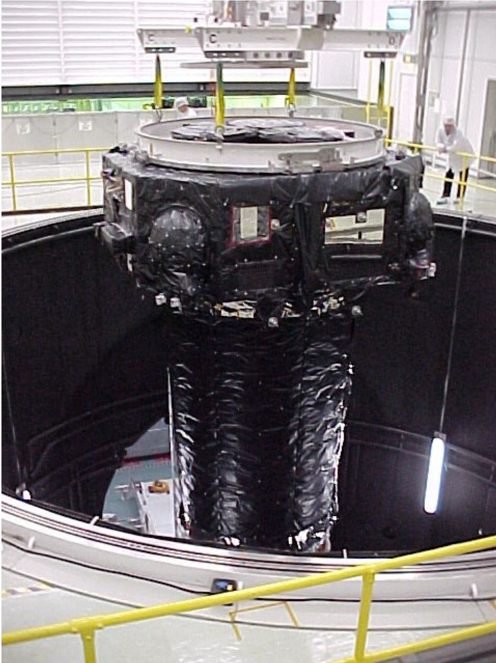
The XMM lower module emerging from the Large Space Simulator in ESTEC in 1999. Credit: ESA
