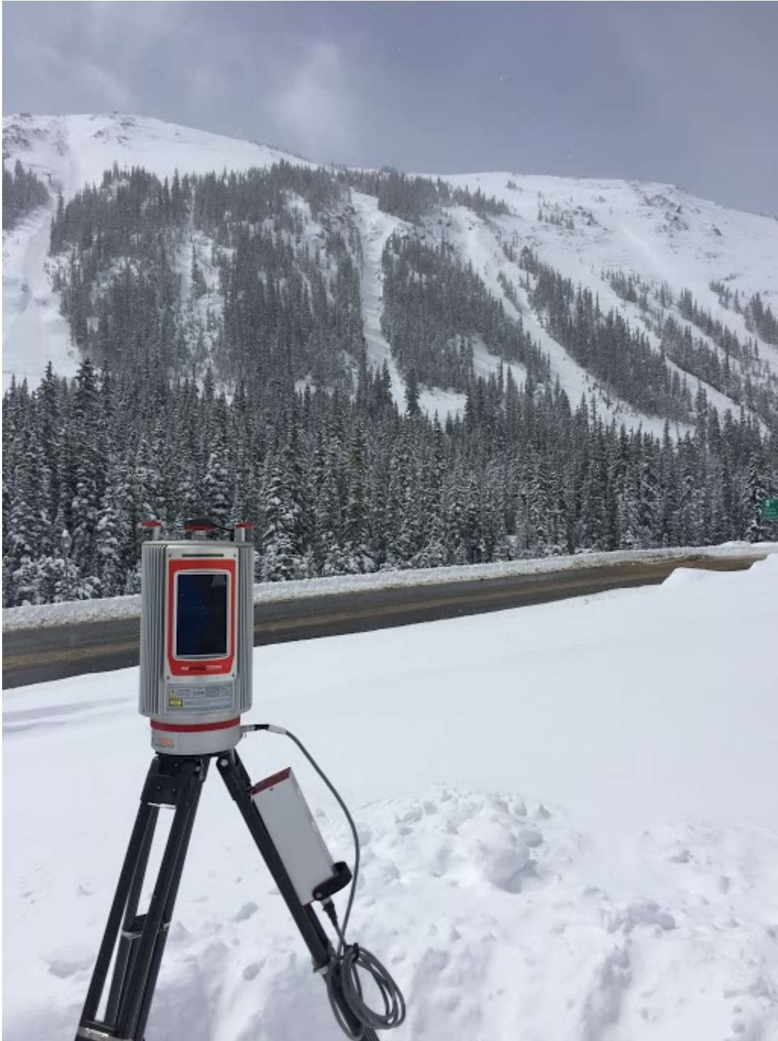
Researchers use this laser-scanning (lidar) instrument to map snow depth at very high resolution. Credit: J. Deems, NSIDC/CIRES/CU
