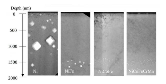
An electron microscope reveals the radiation-induced cavities inside samples of pure nickel and alloys. The cavities in nickel-cobalt-iron and nickel-cobalt-iron-chromium-manganese alloys are 100 times smaller than those in pure nickel. Credit: Wang Group, University of Michigan
