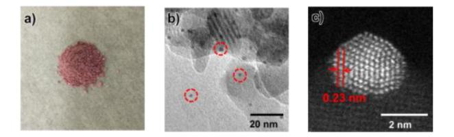
Figure: a) Gold nanoparticle catalyst (Au/HAP-NC), b) Images of gold nanoparticles (black dot in red circle) through Transmission Electron Microscope, c) Annular Dark Field of gold nanoparticles through scanning electron microscope. Credit: Osaka University
