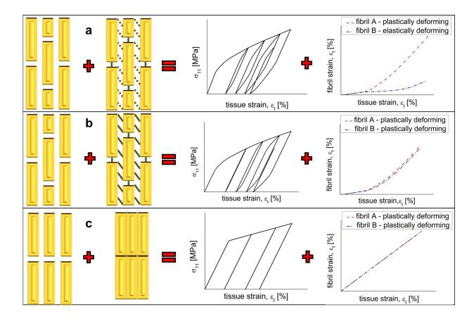
(a) Staggered fibrillar configuration and damageable mode II interface are responsible for hysteretic stress strain curve and heterogeneous fibrillar deformation. (b) The inclusion of staggered configuration and undamageable interface leads to hysteresis and homogeneous fibril deformation. (c) Aligned fibrillar configuration and no interface lead to no hysteresis and homogeneous fibril deformation. Credit: QMUL
