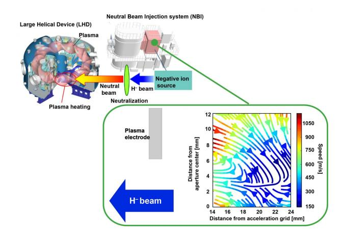
Negative hydrogen ion flow changes its direction toward the electrode aperture when the beam is extracted. Credit: Dr. Masashi Kisaki
