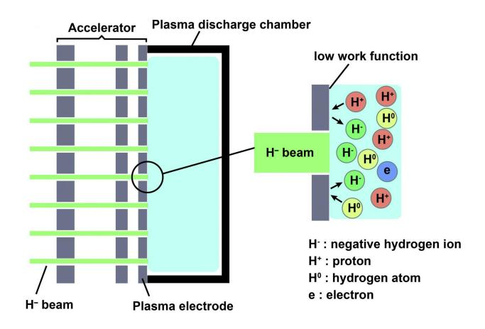
The work function of the electrode surface becomes low with introduction of the cesium into the ion source, and the negative hydrogen ion production is enhanced. Credit: Dr. Masashi Kisaki
