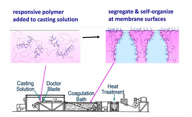
Schematic description of the non-solvent induced phase separation (NIPS) membrane casting in the presence of an amphiphilic responsive copolymer additive. Credit: *Technology*
