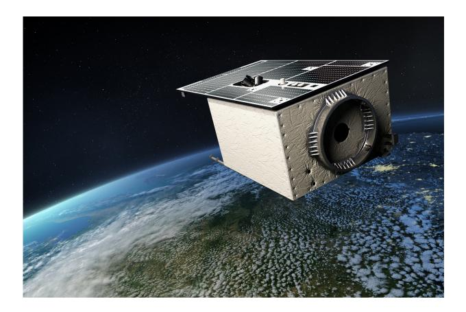
EnMAP is a German hyperspectral satellite mission for earth observation. Imaging spectrometers measure the solar radiation reflected by the earth's surface from visible light right through to shortwave infrared. These allow statements to be made regarding the state of the earth's surface and any visible changes. The mission is due to be launched in 2018 and will continue for five years. Credit: DLR CC-BY3.0
