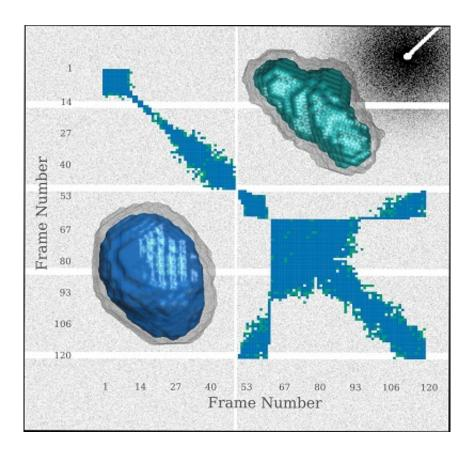
SAXS envelopes of Glucose Isomerase generated from frames collected early (bottom left) and late (top right) in the experiment. Credit: Brooks-Bartlett et al
